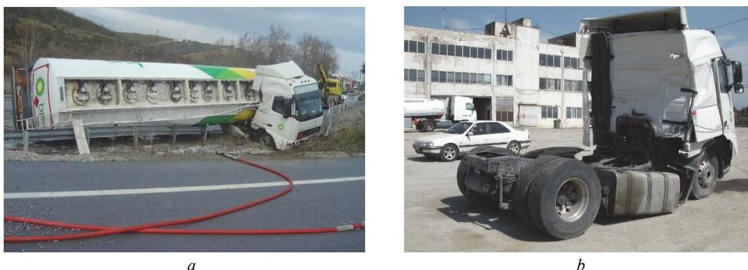
Figure 2. The semitrailer loaded with 38 m<sup>3</sup> unleaded gasoline, after an airborne 180 degrees travel rests on its right side on the road guardrails. The road tanker before the accident was travelling downhill in the reverse direction from this laying in picture (a) The tractor's chassis was completely damaged during the accident (b)
