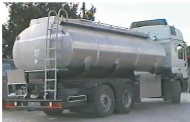
Figure 8. Three-axle 26T gross-weight road tanker:
